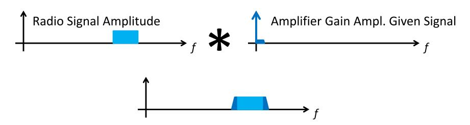
Spectrum is Broadened ... Some energy leaks into Adjacent Channels
