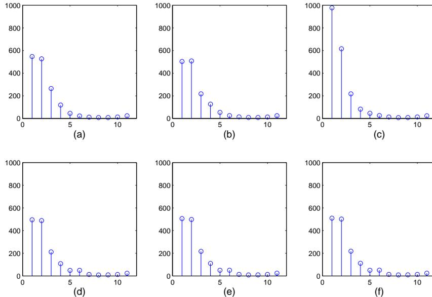
Fig. 4. Robust PSD features. (a)-(c) are the original PSD features for three segments of the data, while (d)-(f) are the corresponding stabilized PSD features. The x-axis denotes the frequency bins and y-axis shows the average power spectral density.
