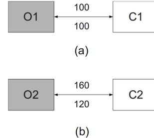
Fig. 1. Example state models used to generate ion-channel signals in QUB. Model (a) is used to generate a signal in the absence of an analyte and model (b) in the presence of an analyte with rate constants (100,100) and (160,120) respectively.
