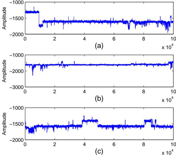
Fig. 3. Experimental data obtained from the sensor array with varying baseline current and noise levels. The x-axis denotes the sample index and the y-axis the signal amplitude.
